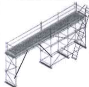
Figure 35 Knee Bracing
