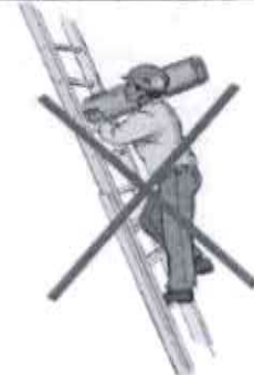
Figure 103 Wrong Ladder Usage
